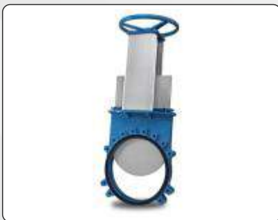
Knife Gate Valves: Size: 6mm to 300mm (1/4" to 12") • Body & End Piece: Cast Steel, Stainless Steel etc • Ratings: 150# to 600# equivalent in BS10, DIN etc • Seat Material: PTFE, Teflon, CFT, GFT, Metal Seated etc.
