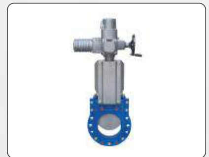
Knife Gate Valves: Size: 6mm to 300mm (1/4" to 12") • Body & End Piece: Cast Steel, Stainless Steel etc • Ratings: 150# to 600# equivalent in BS10, DIN etc • Seat Material: PTFE, Teflon, CFT, GFT, Metal Seated etc.
