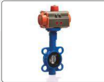
Butterfly Valves: Sizes- 1/2 " to 20" • Body Material- WCB/CF8/CF8M/MS • Disc Material: SS304, SS316, SGI, Teflon Coated/Rubber Line • Pressure Range - Upto 20 Bar • Seal Material- PTFE, Teflon, EPDM, Silicon, Viton etc
