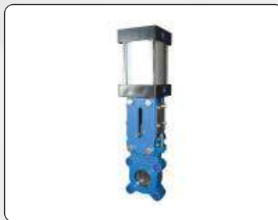
Knife Gate Valves: Size: 6mm to 300mm (1/4" to 12") • Body & End Piece: Cast Steel, Stainless Steel etc • Ratings: 150# to 600# equivalent in BS10, DIN etc • Seat Material: PTFE, Teflon, CFT, GFT, Metal Seated etc.
